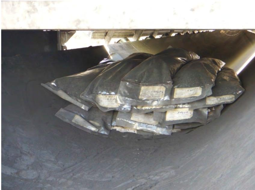
**Figure 2: Typical loading of samples in beam path of a through-belt PGNAA gauge.**
