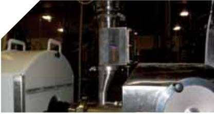
**MoistScan**<sup>®</sup> MA-700 analyser installed on the in-feed to a hydrator at a snack foods factory. The analyser measures the moisture in a mixture of polenta and rice. Data from the **MoistScan**<sup>®</sup> directly controls moisture addition to the hydrator to ensure the product meets quality specification.
