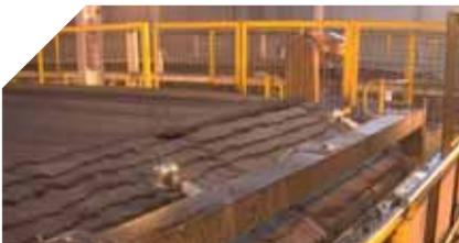
**MoistScan**<sup>®</sup> MA-600 installed on a horizontal belt filter at a coal wash plant. The MA-600 has 3 sets of antennae across the belt. The analyser calculates average moisture across the belt which is used to control belt speed and flocculant addition.
