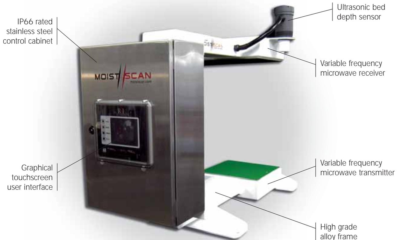
Our patented **MoistScan**<sup>®</sup> dual measurement multi-frequency microwave generator measures attenuation and phase shift of the microwave signal at discrete pre-defined frequencies.
