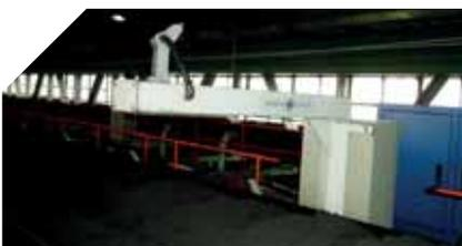
**MoistScan**<sup>®</sup> MA-500 installed on the coal receival belt of a power plant. The MA-500 is used in conjunction with an online elemental analyser to determine the total dry ash percentage and sulphur content of the received coal.
