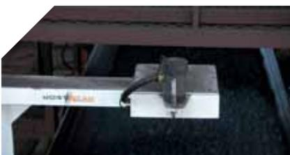
**MoistScan**<sup>®</sup> MA-500HDi measuring moisture content of iron ore pellets at a shipping port. The analyser is used to calculate the total dry tonnage as the product is loaded onto the ship.
