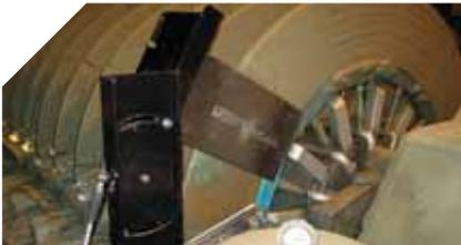
**MoistScan**<sup>®</sup> MA-600 installed on a vertical disk filter at a copper processing plant. The analyser measures the moisture in filter cake. Data from the **MoistScan**<sup>®</sup> controls the vacuum pressure of the filter plates to produce a filter cake within a tight moisture specification of 7-8%.
