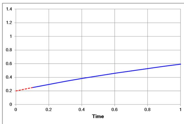
Figure 2. Backward extrapolation of the variogram to estimate the measurement variance.
