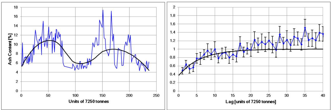
Figure 8. Data, detrending and z-score variogram for coal C.
