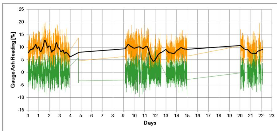
Figure 10. On-line analyser data for low ash coal showing detrending and deviation values from the trend.
