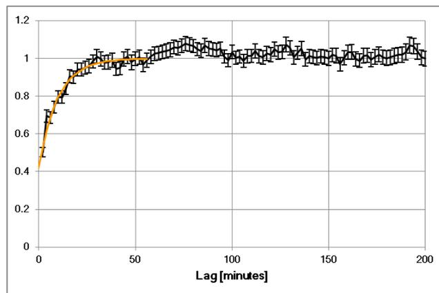
Figure 13. Variogram for high ash coal derived from on-line analyser z-score data.
