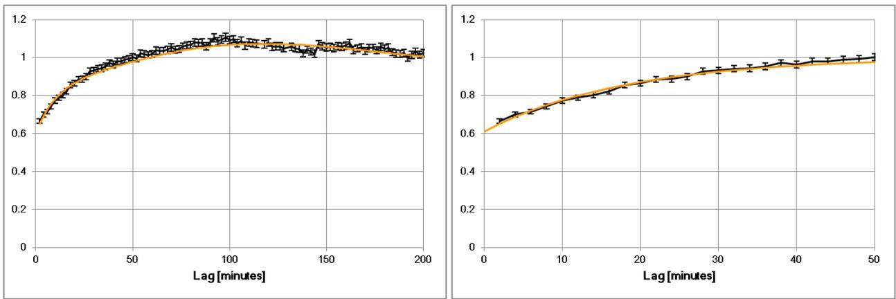
Figure 11. Variogram for low ash coal derived from on-line analyser z-score data.
