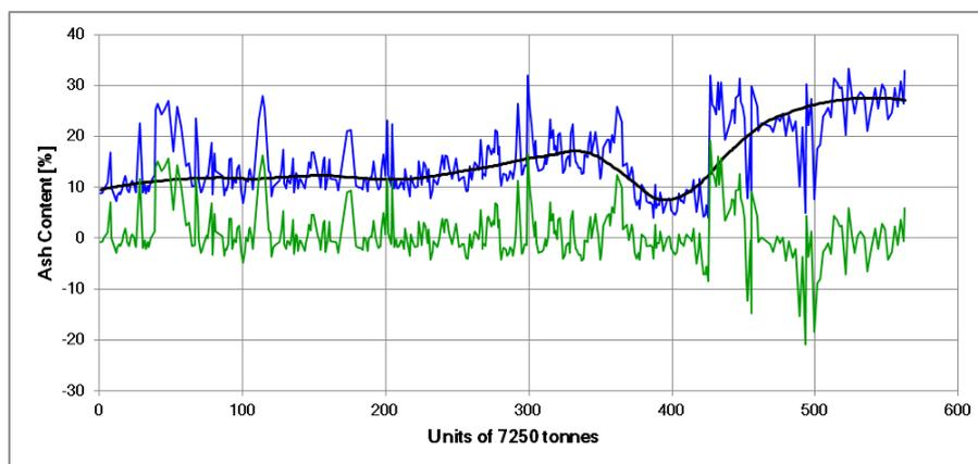
Figure 3. Ash content of coal type A as a function of tonnes of coal sampled.
