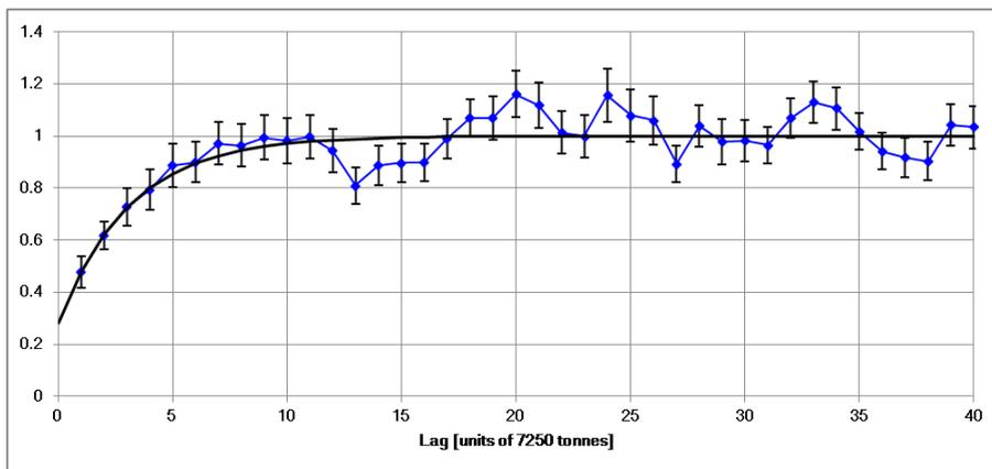
Figure 6. Variogram for coal A as sampled using z-score values, with a fitted exponential variogram. The intercept value is 0.284 from the fit.
