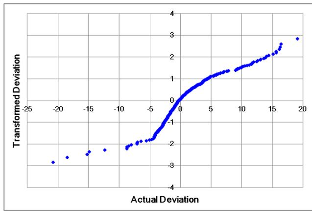
Figure 4. Transformation of deviation data to a standard normal distribution (Q-Q plot)
