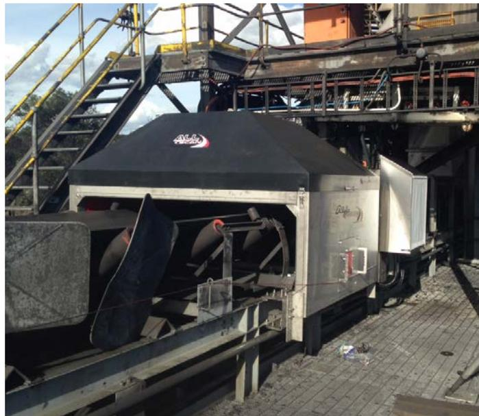
Figure 9. Installation of an Allscan gauge for measurement of coal ash.
