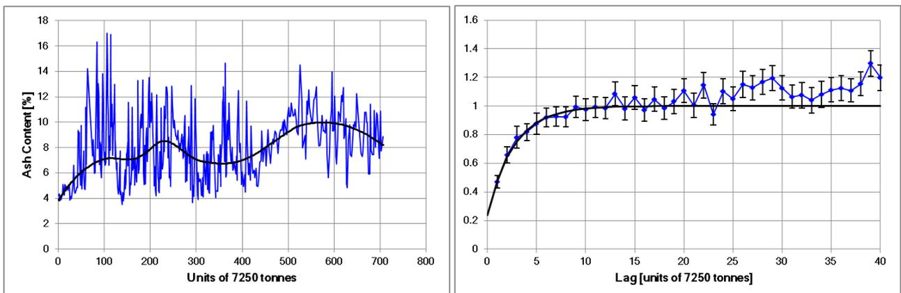
Figure 7. Data, detrending and z-score variogram for coal B.
