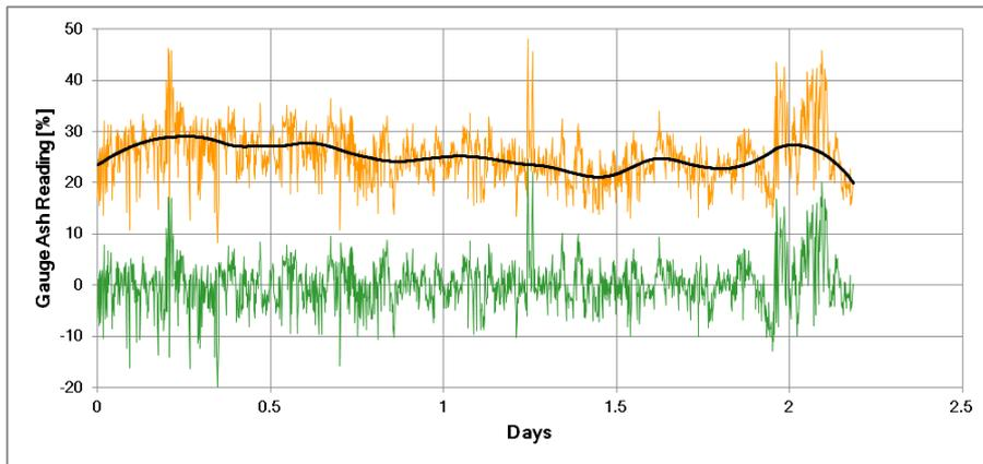
Figure 12. On-line analyser data for high ash coal showing detrending and deviation values from the trend.
